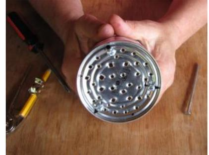
**2d. Make the secondary air holes.** Take your 15 oz can and punch 8 evenly spaced holes around the top rim.
