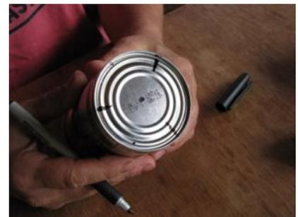
**2b. Install the legs.** Take the hammer and nail and lightly punch 3 small holes in the can bottom near the points on the rim. Install a machine screw in each hole to make the legs of the pyrolytic combustion chamber.
