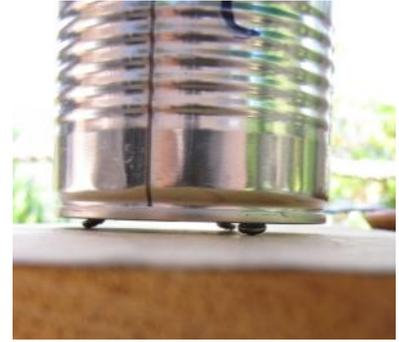
You now have a can with nail holes (for primary air) in the bottom, can punch holes (for secondary air) around the rim, and 3 feet made of screws. You can adjust primary air by changing the height of the screws. For extra fun, try making another can with a different primary air hole pattern and see what happens.
